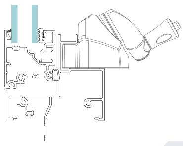
Touchstone Awning (horizontal opening) and Casement (vertical opening) windows are designed to give your new or renovated home a distinctive style as well as ventilation control. Their appearance is sleek and flush with your external walls because of the sash profile on the window's exterior.
